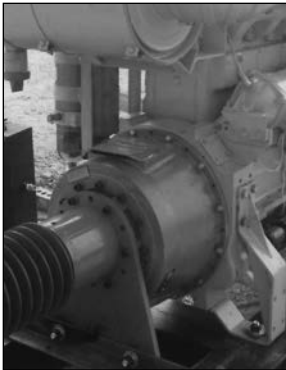
Wichita PTO mounted on Caterpillar diesel engine.
