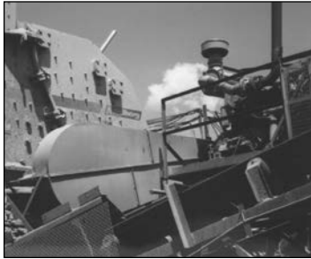
Wichita 15-1/2" mechanical PTO provides long service life for Cummins 855 diesel on rock crusher.
