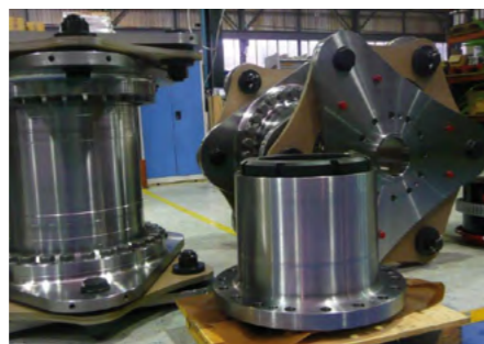
Jaure JHC-F-320 in combination with Lamidisc 1300-6 for Water Jet Drive
