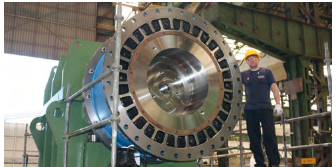
Max-C high elastic coupling
