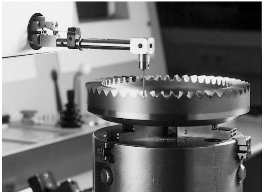
Computerized mapping of gear tooth profile
