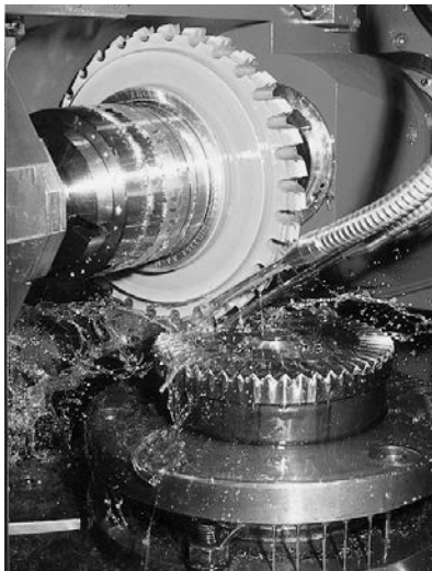
CNC machining of a PowerTRUE right-angle gear
