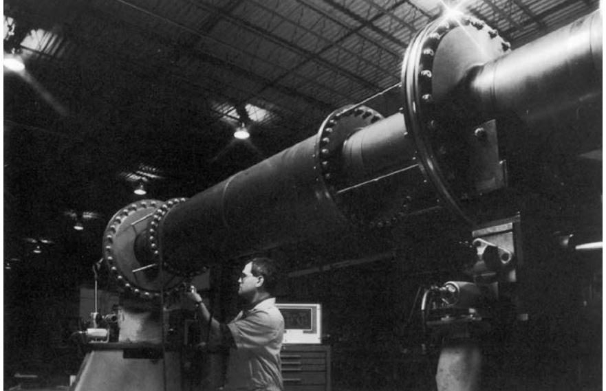
Assembly balancing of a S23-10 Ameriflex coupling for the LM-6000 gas turbine
